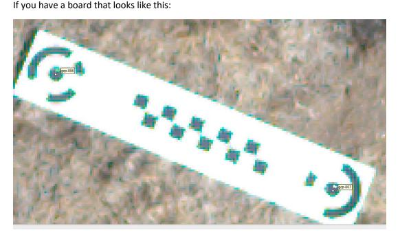
You'll treat it as two normal GCP points and a scale bar. Complete the marker placement for all of the other GCPs in the scene before pinning the GCPs on the scale board.
