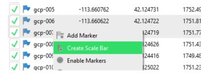
The scale bar will appear below the markers in the Reference pane. In the Distance section, add in 1.0m (this will depend on the scale so check with whomever collected the data).
