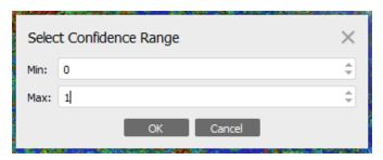
The remaining point cloud is made up of points that have a confidence of 1.
